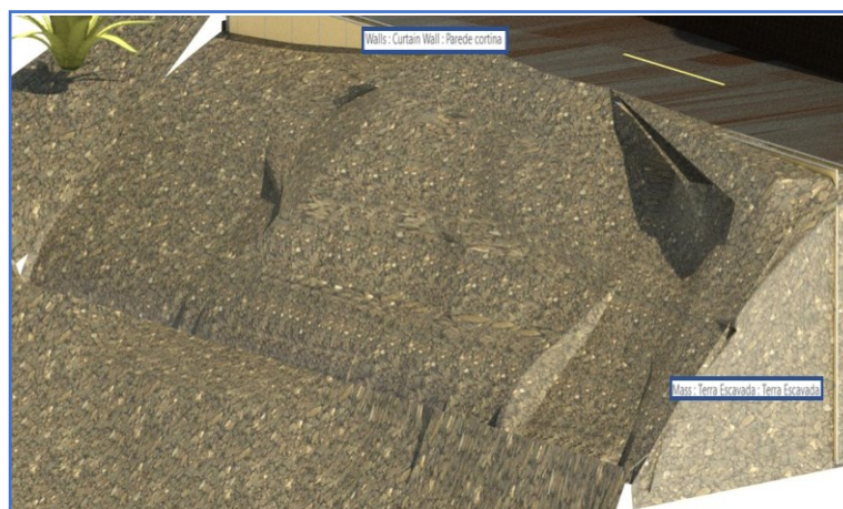
Figure 5. Mass In-place element representing the excavated soil.
